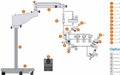
Base Column 1<sup>st</sup> arm 2<sup>nd</sup> arm Focusing unit Joint arm Microscope body 45° Inclined adapter Parallel binocular tube 12.5x Eyepiece F=200 mm objective lens Foot switch **Optional accessories**
